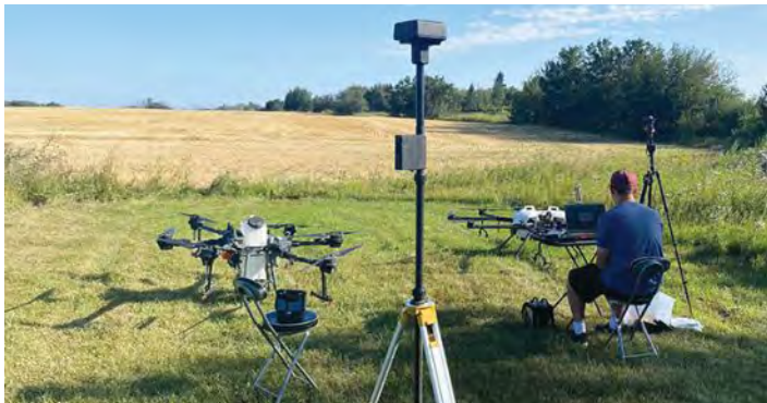
Fig. 5. Preparing the sprayer drones for testing and calibration. Image: Landview Drones.
