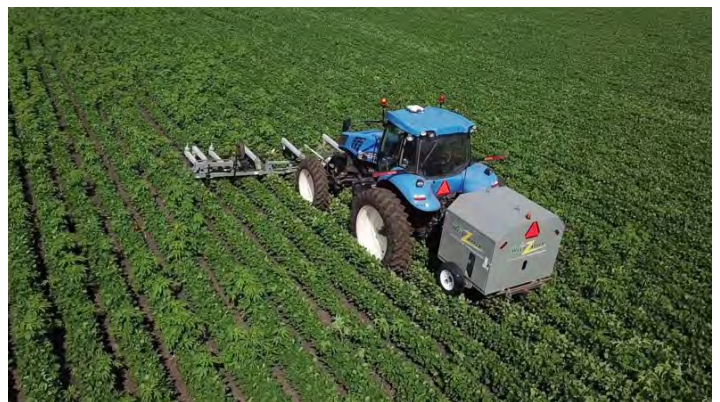
Fig. 8. The Weed Zapper uses electricity to zap weeds growing above the crop canopy. Image: Crop Fertility Services.
