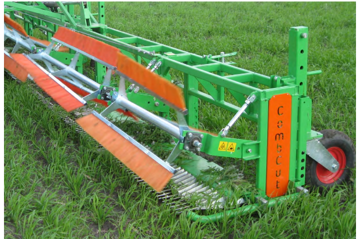
Fig. 7. CombCut weeder cuts the rigid stems of the thistle while having minimal damage to the flexible cereal crop. Image: Katherine Stanley.
