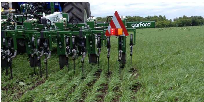
Fig. 6. Interrow cultivation supported by camera guidance and side-shift technology. The camera detects the crop row and then uses side-shift technology to position the tillage equipment between rows and avoid hitting the crop. Image: Joanne Thiessen Martens.
