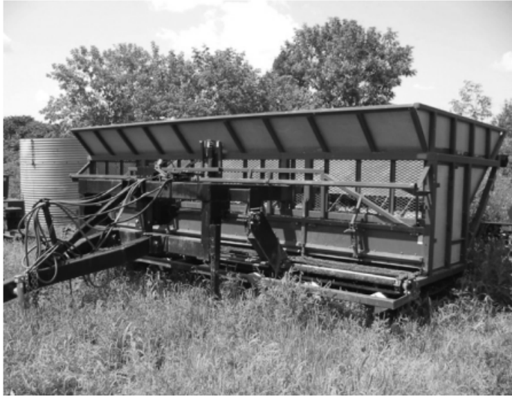
Figure 22. Custom built manure spreader to allow low rates of compost to be applied. Quebec.
