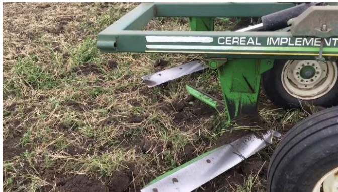
L: wide blade cultivator used for summer fallow tillage; leaves residue on surface. R: field bindweed.
